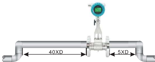
Two Square Bends At Different Plane
