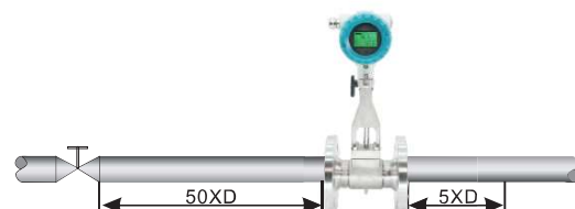
Regulating Valve, Half-open Gate Valve
