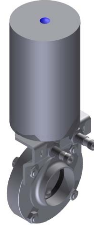
Figure 4: Butterfly valve type Classic with pneumatic actuator and end position feedback
