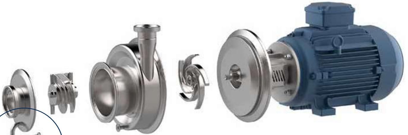
The clamp casing and seal design allows quick disassembly for inspection, cleaning and maintenance.
