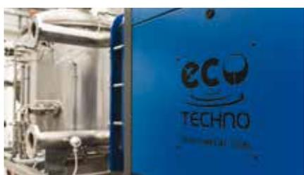
**Low temperature evaporators (heat pump)**
