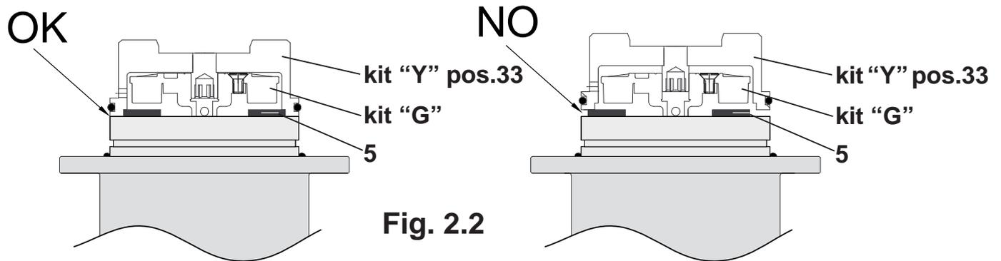
2.06) Position the top casing and secure it with the twelve screws **pos. 57** and the nuts **pos. 58**, using a dynamometric spanner.
