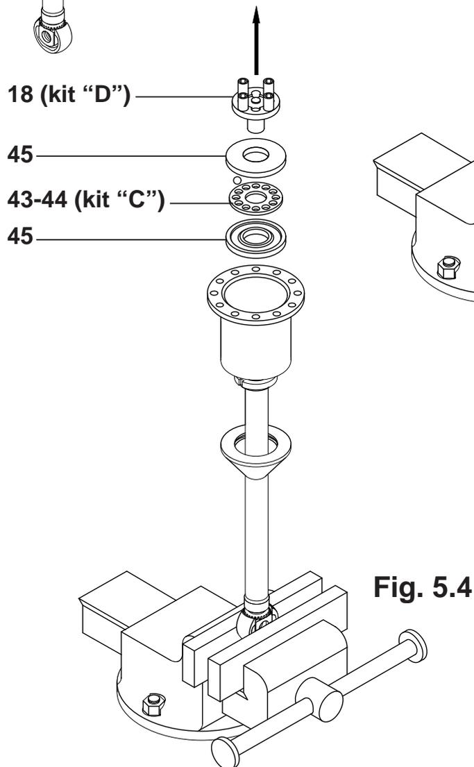
5.04) Slide the complete internal rod out “A” (Fig.5.5)
