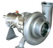
Open impeller centrifugal pumps with a separate shaft a support frame containing oil-grease lubricated bearings.Wetted parts in CF-3M 1.4404 / AISI 316L stainless steel, investment cast and electrochemically polished.
