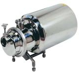
Self-priming sanitary pumps. A close coupled design with independent shaft support and standard IEC motors. The ability of these pump to maintain a vacuum under varying suction conditions, makes them ideal for applications where the incoming liquid contains gas or air, such as vessel scavenging, the handling of foaming liquids or where the suction pipe is only partially flooded. All CF-3M 1.4404 / AISI 316L stainless steel parts.
